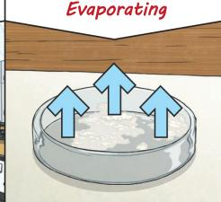
The **liquid** changes into a gas, leaving the solid particles behind in the dish·
